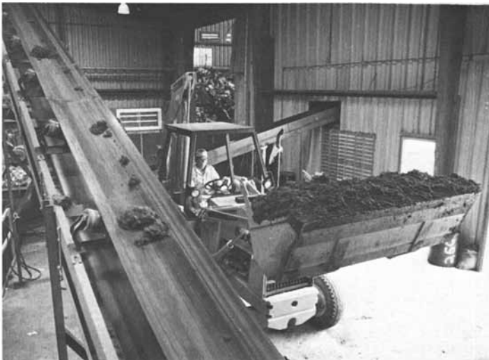
Figure 5. Front loader scooping sludge cake
