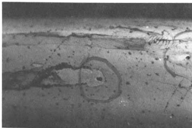
Figure 6. Pitting damage of Bellows Seal on reactor
