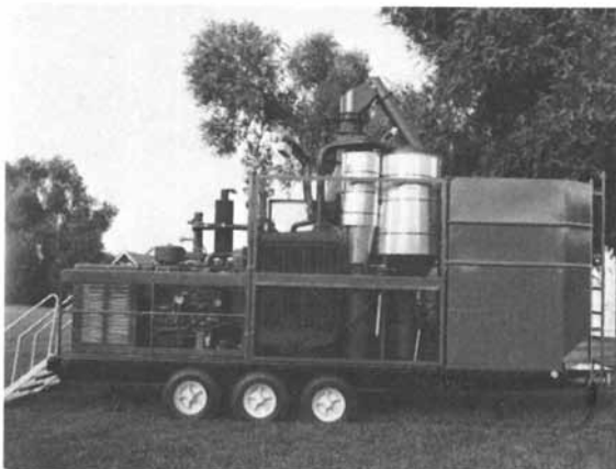
Figure 5. Gas producer system showing insulated cyclone and filters
